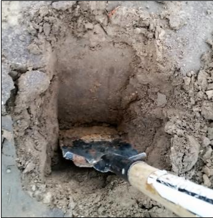
Fig 38. No sloppy clay for at least 30cm depth in scald at end of the overflow area
