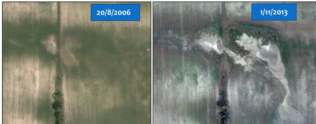
Fig 27. Google earth comparisons of main seep area showing extensive spread of scald
