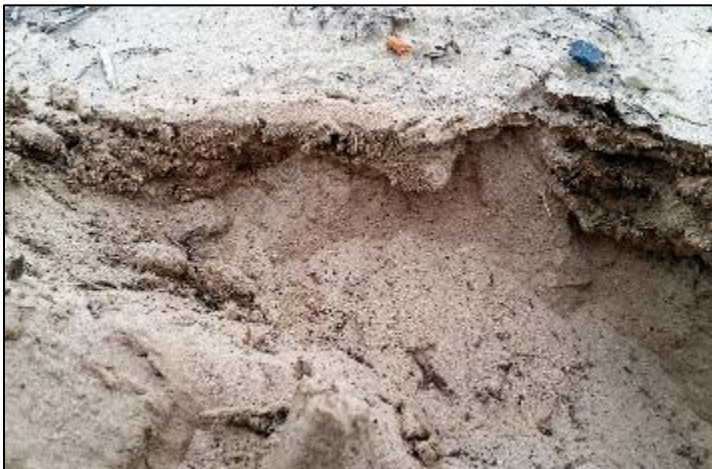
Fig 41. Dry sand under surface sand crust, Sandhill, May 11, 2016
